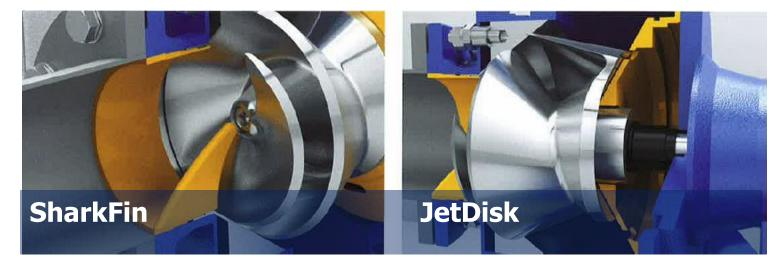
The **SharkFin** is located in the pump suction port and provides an optimized deflection of the incoming solids and fibrous material toward the centre of the impeller. This reduces solids settling and clogging, resulting in significantly less downtime.
